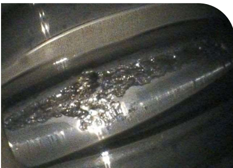
Figure 10: Spalling damage initiated from surface damage at the dedendum of a gear tooth.
