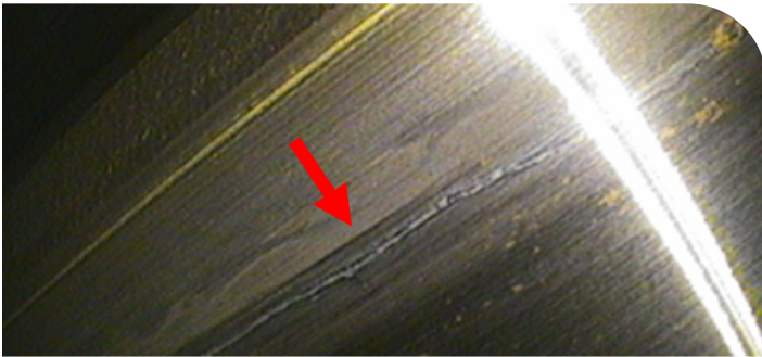
Figure 30: Scratch on gear tooth
