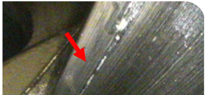
Figure 31: Straight-line micro pitting
