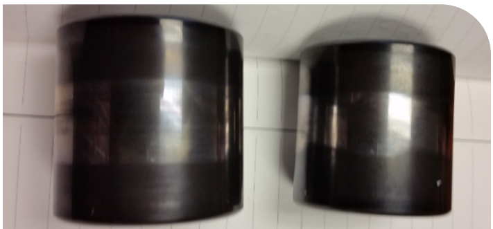
Figure 32: Black Oxide Coating worn away, depicted via bore scope on the left, and unaided visual on the right
